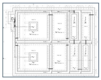
required geotechnical and surveying information from site. The geotechnical evaluation was done locally in South Africa after clay samples were taken on site and shipped to a South African soils laboratory. The design was finalised and drawings were provided to the site engineer and contractor. The construction of the 12,000 m² size pond system was done within a period of 40 days.
